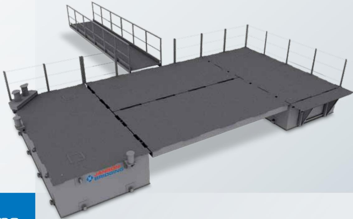
The Janson Couple Pontoons are designed to be transported in standard trucks. They are lowered into the water by crane, using the upper couplers as lifting lugs. Once on the water, because of the simplicity and effectively engineered coupling systems, the pontoons can be quickly coupled without any mechanical assistance from deck level with 2 unskilled operatives positioned on each pontoon.
