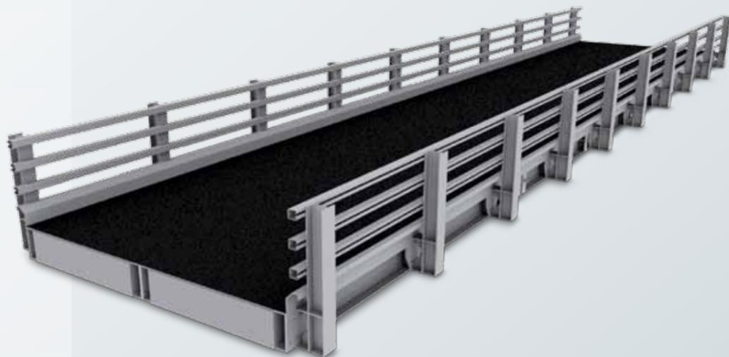
Each Beam Bridge unit has a width of 1.5 or 2.1m. By joining the units side to side, any required road width within the modules can be achieved (3.0m - 3.6m - 4.2m - 4.5m - etc). The outer units can be equipped with parapet rails and kerbs or pedestrian fencing. The units are available in depths of 300mm and 450mm and have an integrated anti-skid surface consisting of epoxy resin embedded with aggregate.
