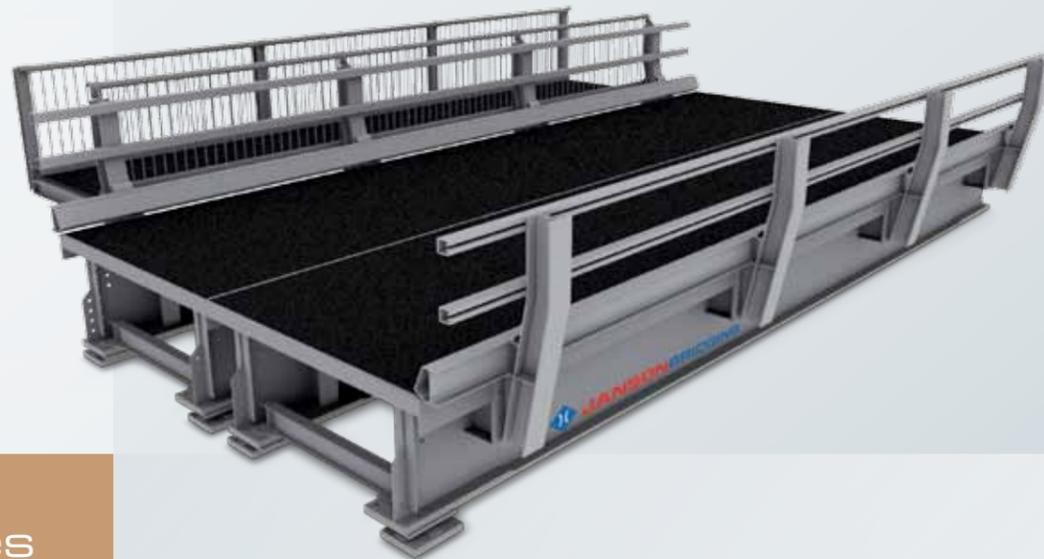
Each unit has a width of 2.5 or 3.5m. By joining the units sideways any required road width within the modules can be achieved (3.5 - 5.0 - 6.0 - 7.0 - etc.). The exterior units can be equipped with parapet rails and kerbs or pedestrian fencing. The units are built from steel trusses with integrated steel trough decks which have an integrated antiskid surface consisting of epoxy resin embedded with aggregate.
