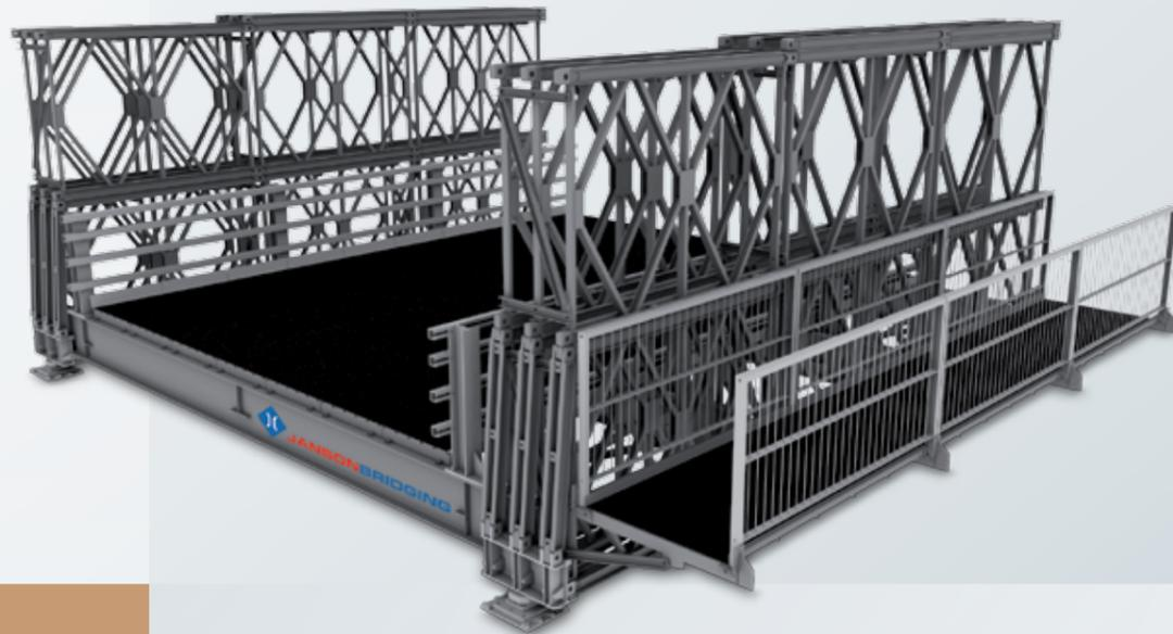
Janson's Panel Bridge system is a modular system where basic components, the modular rectangular panels with 3.048m length, are pinned and bolted together to form the bridge's longitudinal trusses. The trusses can be assembled in various constructions to form girders where strength is tailored to suit the span and loading of the individual bridge.
